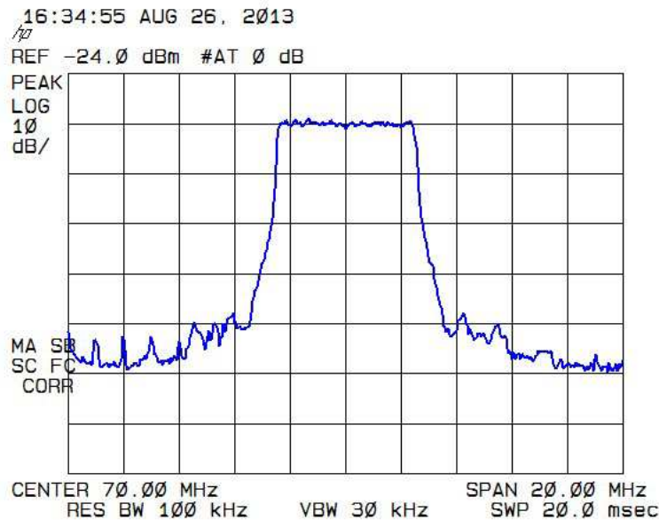
Figure 1 Measured OFDM spectrum
