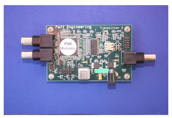
The evaluation board provides a means of testing the IP, utilizing an Altera Cyclone 3 FPGA and Texas Instruments DAC904 converter, clocked at 160 MHz. A bandlimited BPSK signal with root raised cosine filtering (25%), centered at 70 MHz, is provided at the output port., Digital clock and data is applied to the BNC input ports to establish the data rate and the transmit bit pattern.
