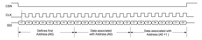
The format of writing data to the Evaluation board is illustrated above. Data on the SDI line is transferred on the positive transition of CLK when CSN is active low. The CSN line may remain low for transfers of 1 to 8 bytes of data. The most significant bit is sent first in each byte transmission. The address increments by one after each byte is written.
